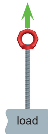
Pic. 4: Only axial loading! No swinging!
