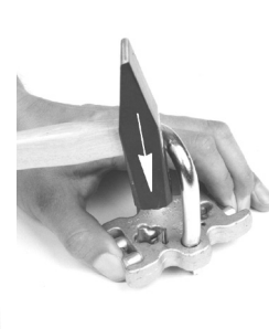
Press locking pins and hammer in a new clamping sleeve.
