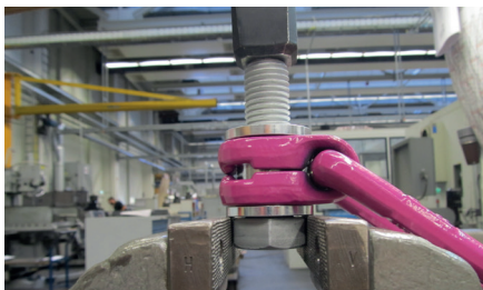
Pic. 5: Dismantling position of the L-VLBG
