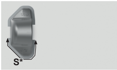
Pic. 1: Weld on welding block 1
