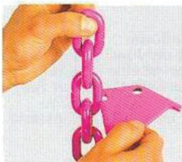
Testing wear of nominal diameter
