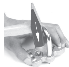
Press locking pins and hammer in a new clamping sleeve.
