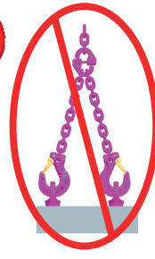
Pic 2: Wrong assembly and usage. Only one load bearing strand is permissible
